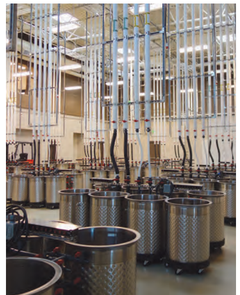
Cypress Semiconductor donated tank controllers that include wireless networked functionality, variable-speed pumpover pumps, Brix sensors, temperature sensors and valve controllers.
